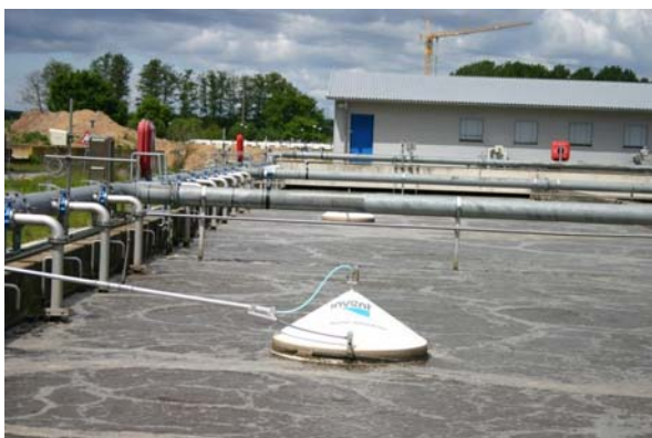
ALPHAMETER ® - Off-gas collection hood on site
