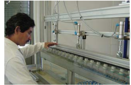
Leakage test of an air distributor
