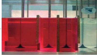
Optimal design prevents short circuit flows and guarantees optimal reactor behaviour.
