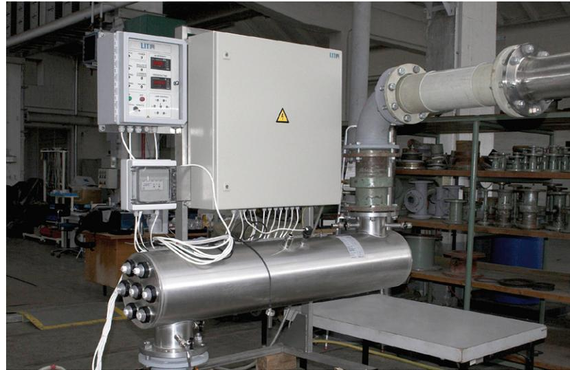
Certification of UV equipment according to ÖVGW standard (Austria)
