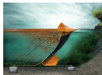
Oil barrier in water
